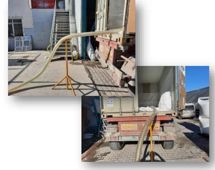
If no hose support is being used, ensure that the hose does not exert any pressure to the valve. Ideal standing is shown at the picture.
